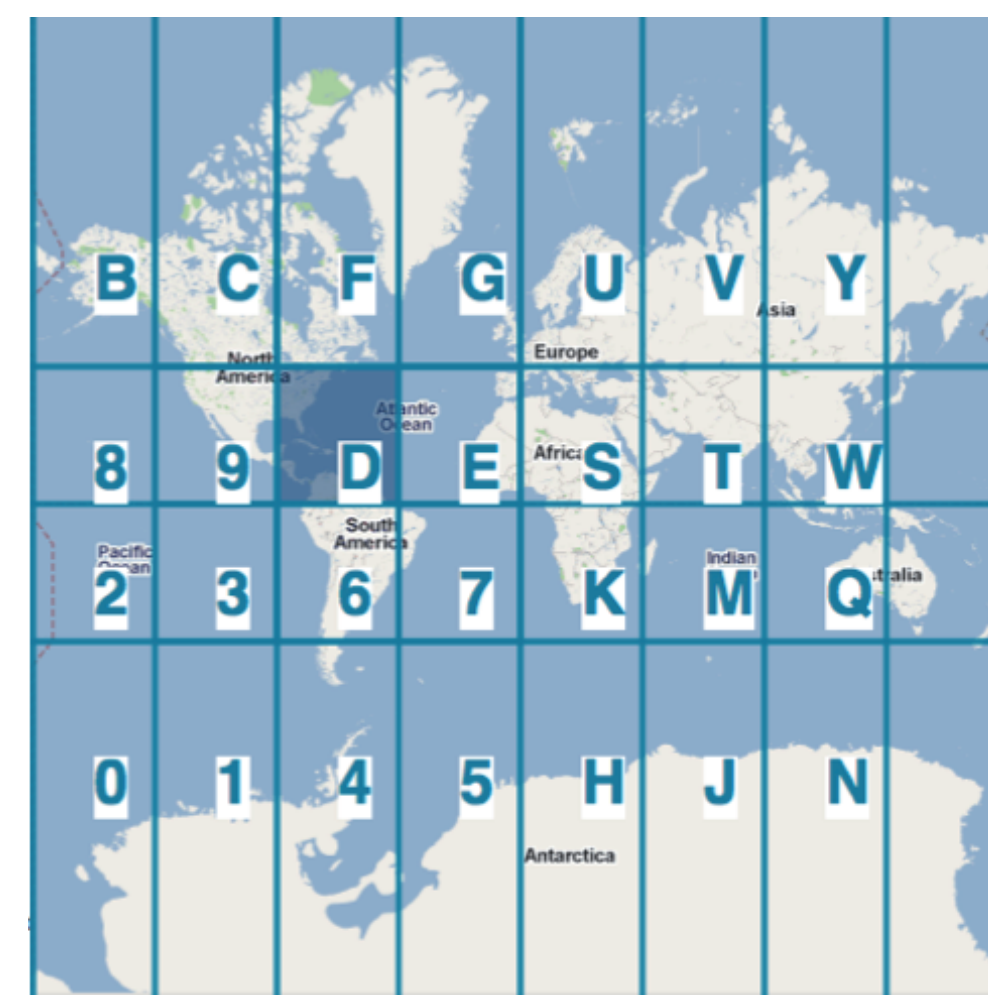
Geohash space decomposition on level 1. The letter „D“ covers parts of the Americas
